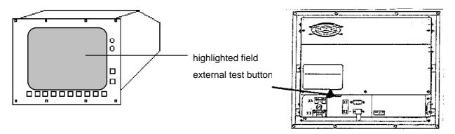
If the VDU generates this highlighted field, the PLC graphics board in the logic unit is probably defective. If however, the VDU remains dark after the test button was pressed, the VDU is defective and must be exchanged.
