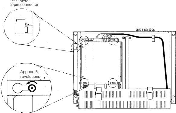
Slide out the power supply unit to the right and insert the new power supply unit.
