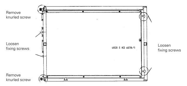
f) Lift out the processor board; exchange the EPROMs, if required (see section 21.8). Insert the new board.
