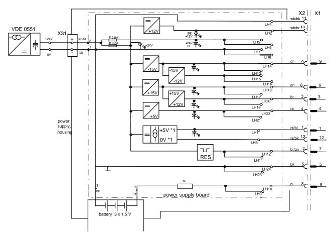
X2: connector (12-pin) of connecting cable "power supply <-> processor board"
