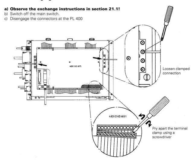
d) Unscrew the cover of the PL 400 and disconnect the cable to the PLC graphics board from the PL 400.
