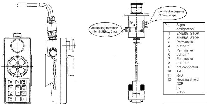
The assignment of the handwheel keys depends on the version.
