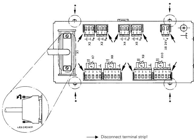
D-Sub connector Loosen knurled screw
