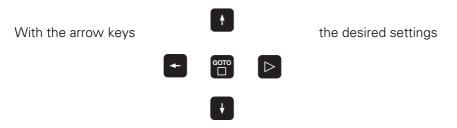
(operating mode, baud rate, interface allocation) can be selected and set according to your requirements by pressing ENT.
