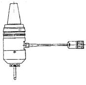
**APE 110** Id.No. 230 465 -- for **TS 111 APE 510** Id.No. 227 590 -- for **TS 511 APE 511** Id.No. 237 586 -- for **TS 511** with additional connector for a second SE 510
