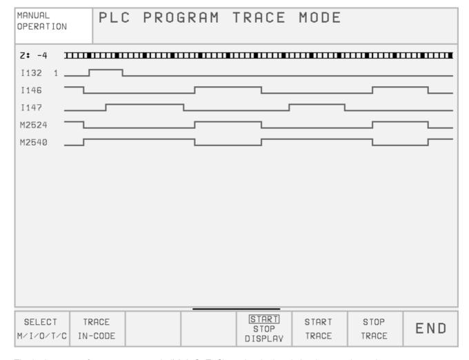
The logic states of up to 16 operands (M, I, O, T, C) can be depicted simultaneously on the screen. 1024 PLC scans can be traced.
