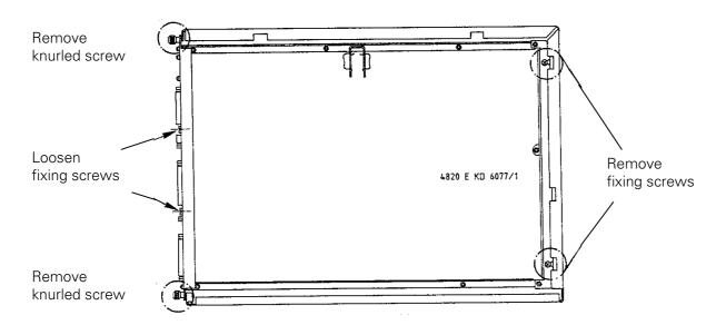
f) Lift out the PLC graphics board and insert the new board.
