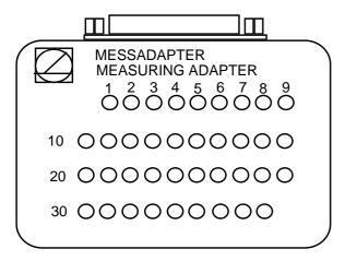
The measuring adapter can be used to test the inputs and outputs of D-Sub connectors (9-pin to 37-pin). On the following page the adapter cables are shown that are required for the different connectors.
