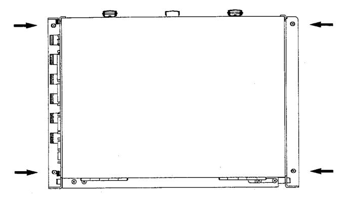
d) Remove the old logic unit and insert the new logic unit.
