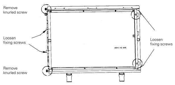
f) Lift out the CLP board; exchange the EPROM, if required (see section 21.8). Insert the new board.
