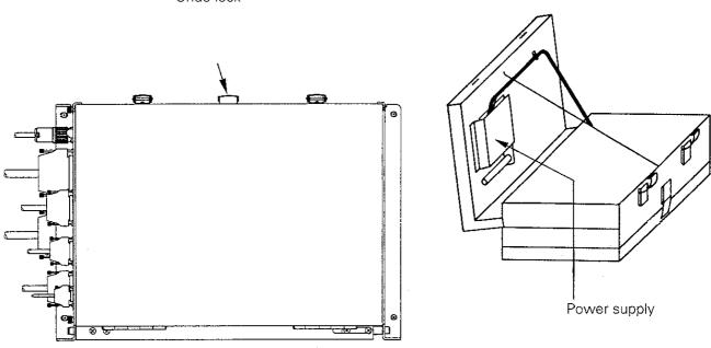
d) Disengage the connection to the power supply unit at the processor board.
