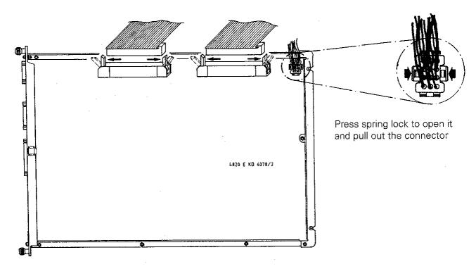
e) Pull the cable harness to the power supply through the housing.
